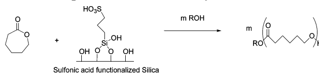
Scheme 2. General Mechanism of ROP of \epsilon -Caprolactone Initiated by an Alcohol
